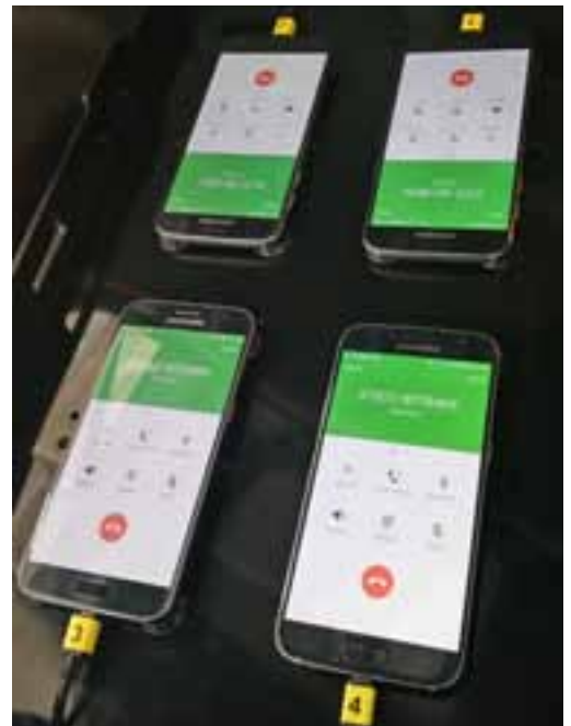
Each box housed four smartphones allowing the simultaneous testing of four mobile operators.
